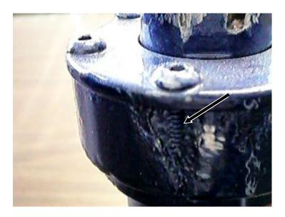
Note the corrosion, exposing one of the Button-head Allen screws-take out of service
