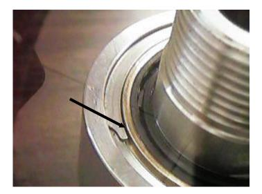
Abnormal retaining ring seat (note the minimal distance between the inside diameter of the retaining ring and the shoulder of the bearing retainer plate)-take out of service
