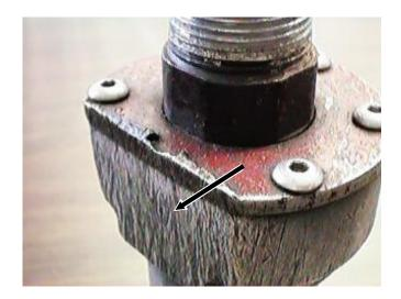
Note the flat-sided wear due to dragging behind a delivery truck-take out of service
