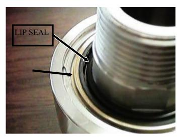
Normal retaining ring seat (note the distance between the inside diameter of the retaining ring and the shoulder of the bearing retainer plate)
