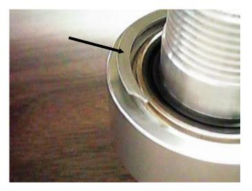
Abnormal retaining ring seat (note the retaining ring tang has come out of the retaining ring groove)-take out of service
